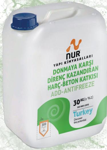
Chlorine-free, liquid, mortar additive which allows cementitious concrete and mortars to be applied in cold and frost weather by accelerating the setting time through increasing hydration temperature of cement and decreasing the freezing point of the water (in 30 kg and 10 kg plastic bins)
